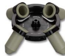
max. volume: 4 x 50 ml conical Order number.: 221.80 V01
