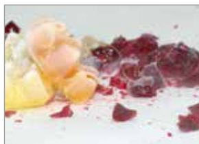
Material embrittled with liquid nitrogen
